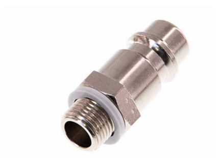
360-Grad Ansicht: KSG 18 NW7 MSV - Coupling plug (NW7,2) G 1/8"(male thread), Nickel-plated brass
